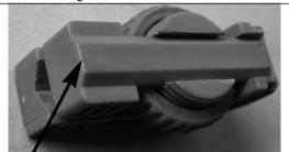
Stepped face upwards for bits of Ø3.5mm to 13mm
